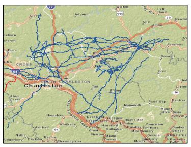
In Figure 6.2.a. above, the blue lines represent gas transmission pipelines. In the case of Kanawha County, all of these pipelines carry natural gas. Capacities vary significantly, as do such specifications as line size, pressure, etc. In most cases, gas flow is heavier during the winter months and is related to home and business heating. The following pipeline operators are active in Kanawha County and manage pipelines carrying natural gas.
