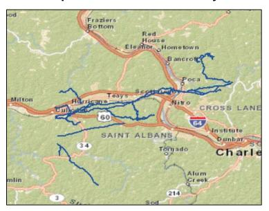
In Figure 6.2.b. above, the blue lines represent gas transmission pipelines. In the case of Putnam County, all of these pipelines carry natural gas. Capacities vary significantly, as do such specifications as line size, pressure, etc. In most cases, gas flow is heavier during the winter months and is related to home and business heating. The following pipeline operators are active in Putnam County and manage pipelines carrying natural gas.
